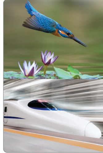
The long, thin shape of the kingfisher's beak (above) influenced the shape of the new and improved bullet trains (below).
