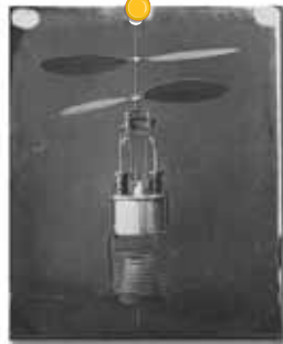
Gustave Ponton D'Amécourt constructed, in 1865, an aerial screw machine that worked by steam.
