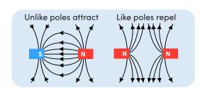
The strength of a force is called its magnitude. The greater the magnitude of a magnetic force, the stronger the attractive or repulsive force between the magnets. The magnitude of a magnetic force depends on the size of the magnets and the distance between them:
