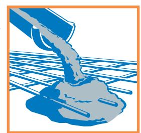
in a kiln to extremely high temperatures—around 2,700 degrees Fahrenheit! This chemical process produces a rock-like substance that is then ground into a fine powder to make the cement. Water and cement form a paste when mixed together, and the paste binds with sand and rock to harden into concrete.
